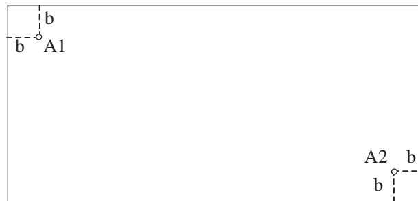
Fig. 4. Positions of acceleration sensors with b = 3 cm.
